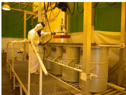
Itrec - Overpack preparation
