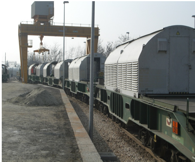
Figure 2: Spent fuel transportation from Caorso NPP
